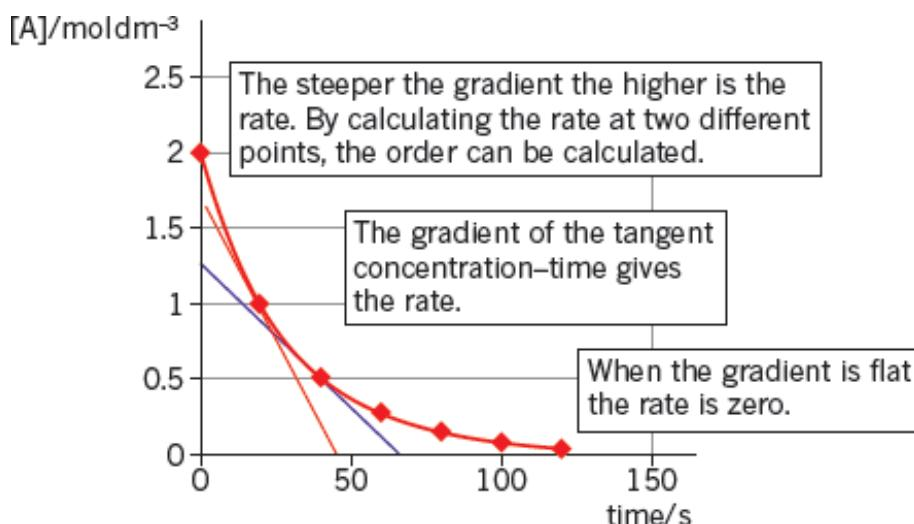
**Note:** When a chemical is listed in square brackets, it just means ‘the concentration of’ that chemical. For example,  $[O_2]$  is just shorthand for the concentration of oxygen molecules.
