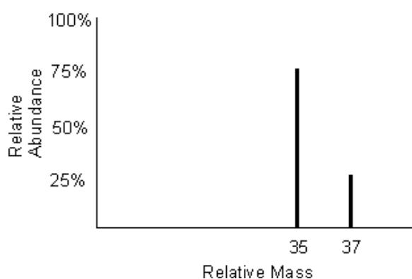
75% of the sample consist of chlorine-35, and 25% of the sample is chlorine-37.
